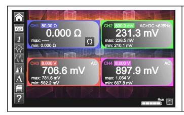
Channel 1 of the *ScopiX* is named CH1. It is used to measure various physical quantities in addition to the signal amplitude measurements, using the appropriate *Probix* accessories. The other channels are voltmeter channels only (or current channels, when used with a *Probix* clamp).
