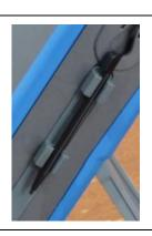
The stylus is stowed in the stylus holder on the side of the instrument.
